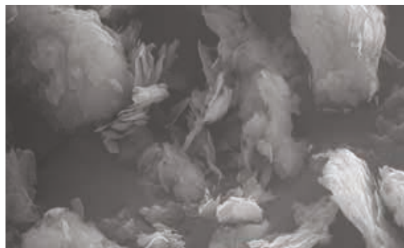
Crys-Talc ® micro-lamellar talc with a high specific surface area showing higher number of nuclei centers
